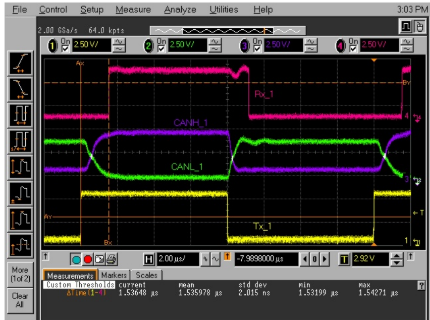
Figure 7. Propagation Delay t_{PD(H)} Between Tx_1 and Rx_1 at 125kB and Cable Length 20m = 1.536 \mu s
