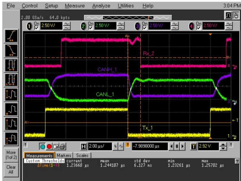
Figure 10. Propagation Delay t_{PD(L)} Between Tx_1 and Rx_2 at 125kB and Cable Length 20m = 1.244 \mu s
