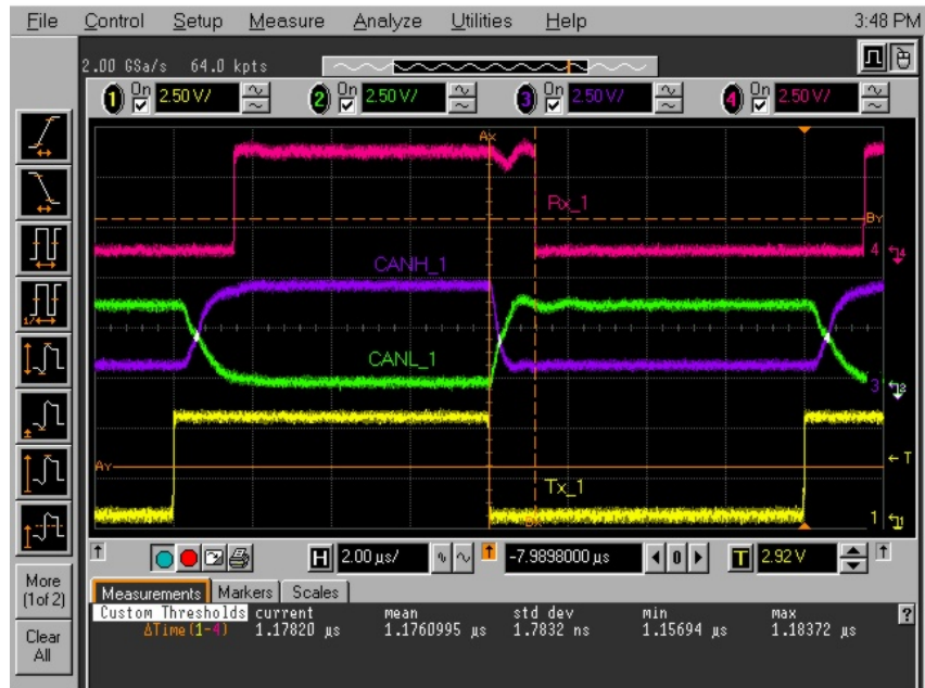
Figure 8. Propagation Delay t_{PD(L)} Between Tx_1 and Rx_1 at 125kB and Cable Length 20m = 1.176 \mu s
